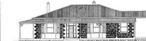
The prototype of the Ladysmith house: the residence of the magistrate, c1890. A core well shielded from the influence of the sun, and a gabled ventilator dormer to release hot air build-up.
