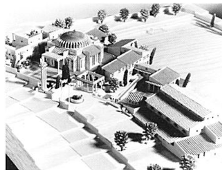
Photograph of the model for the 1988 Design Dissertation. In the realisation, the sides to the dome have become segmented barrel vaults, which butt against the cubical base to the composition, a junction more closely aligned to the precedent, Hagia Sophia, begun circa 532. The bell tower of the dissertation at the entrance has become a campanile, integral with the church. The community centre, foreground left, was built first.
